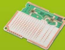
Adaptive Cruise Control with the **HF Board** in cooperation with Bosch
