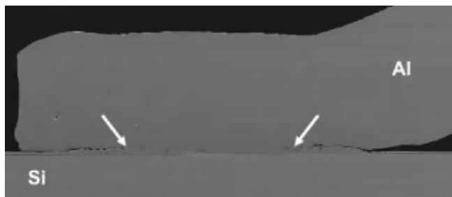
Figure 4: Cracks in a heavy wire bond on an IGBT (silicon) surface. (Source: www.powerguru.org )
